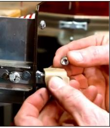
Then attach the handle bracket using the exact same hardware, (2) M6x14mm Button Head Flange Bolts and (2) M6 Nylon Locknuts.
